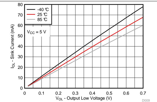
Figure 8. I/O Sink Current vs Output Low Voltage for Different Temperature (T<sub>A</sub>) for V<sub>CC</sub> = 5 V
