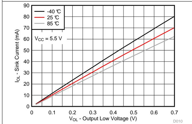
Figure 9. I/O Sink Current vs Output Low Voltage for Different Temperature (T<sub>A</sub>) for V<sub>CC</sub> = 5.5 V
