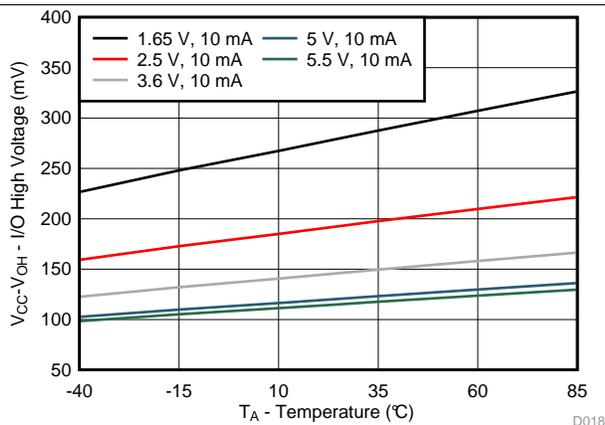
Figure 17.  $V_{CC} - V_{OH}$  Voltage vs Temperature for Different  $V_{CC}$
