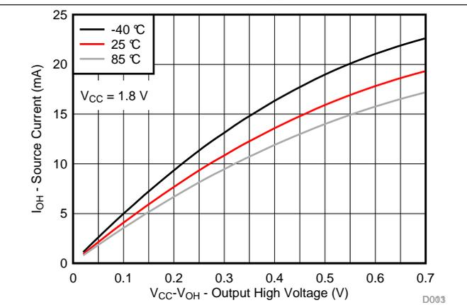
Figure 12. I/O Source Current vs Output High Voltage for Different Temperature (T<sub>A</sub>) for V<sub>CC</sub> = 1.8 V
