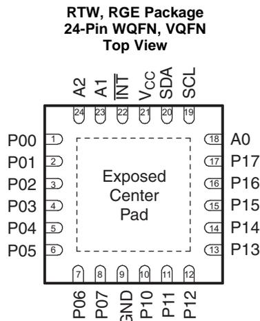
The exposed center pad, if used, must be connected as a secondary ground or left electrically open.
