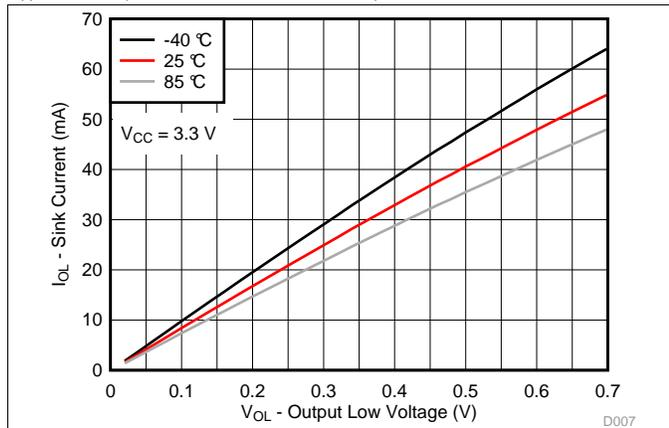
Figure 7. I/O Sink Current vs Output Low Voltage for Different Temperature (T<sub>A</sub>) for V<sub>CC</sub> = 3.3 V
