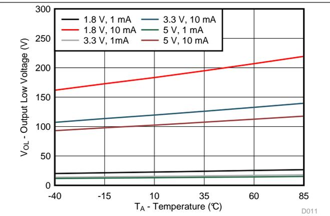
Figure 10. I/O Low Voltage vs Temperature for Different V<sub>CC</sub> and I<sub>OL</sub>
