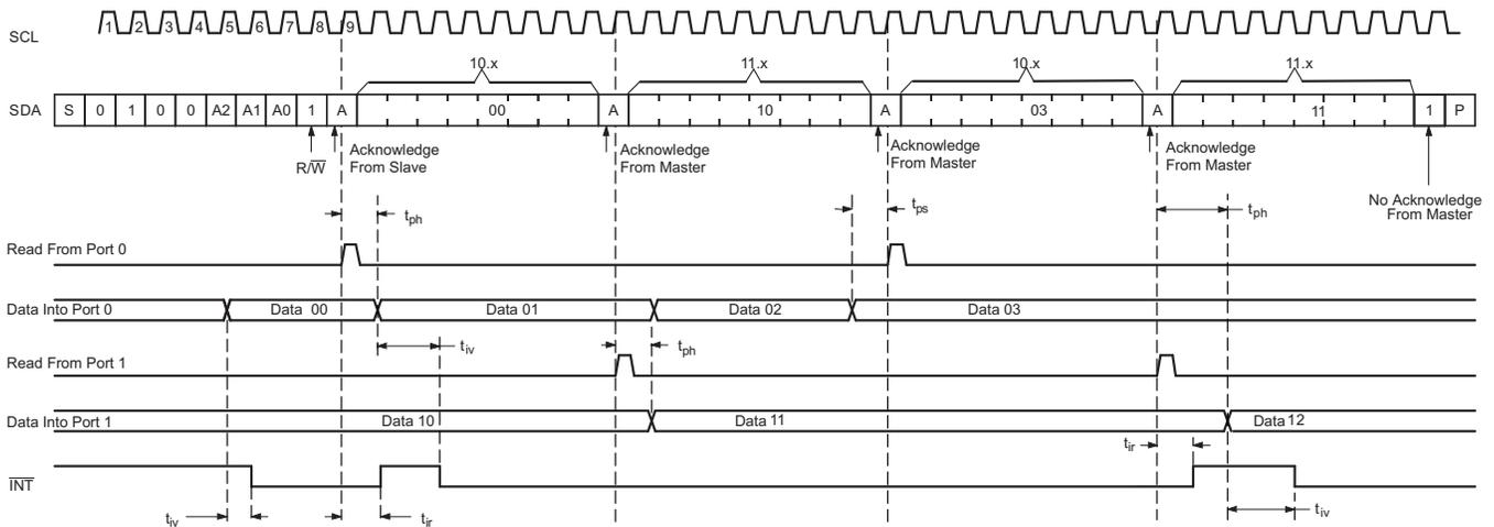
Transfer of data can be stopped at any time by a Stop condition. When this occurs, data present at the latest acknowledge phase is valid (output mode). It is assumed that the command byte previously has been set to 00 (read Input Port register).
