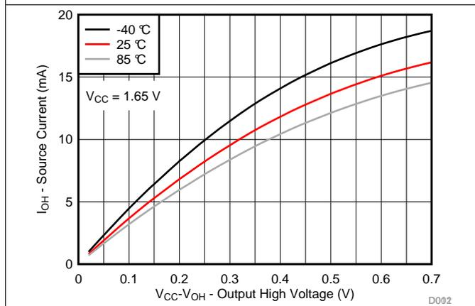
Figure 11. I/O Source Current vs Output High Voltage for Different Temperature (T<sub>A</sub>) for V<sub>CC</sub> = 1.65 V
