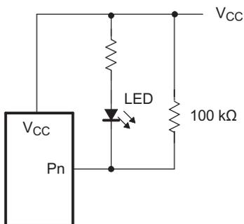
Figure 35. High-Value Resistor in Parallel With LED
