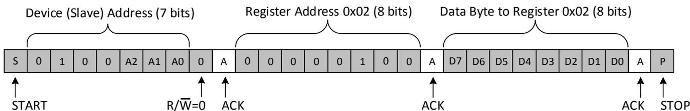
Figure 27. Write to the Polarity Inversion Register
