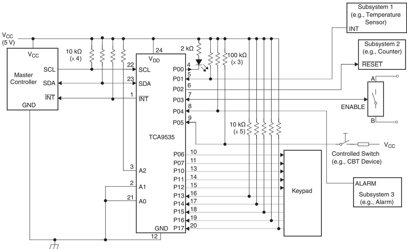
Device address is configured as 0100100 for this example.
