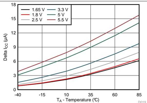
Figure 18.  $\Delta I_{CC}$  vs Temperature for Different  $V_{CC}$  ( $V_I = V_{CC} - 0.6\text{ V}$ )
